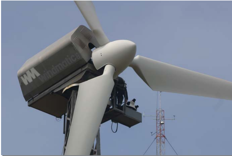
Figure 2 Vindicator® LWS mounted on WindMatic turbine
